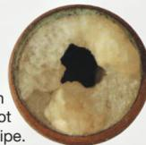
Cross section of a scaled hot water pipe.
